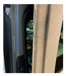
3A) Using a utility knife, start cutting the fabric 1/2" from lip edge. Cut a 1/2" all around the door where there is fabric present.
