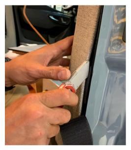
3M) Place 2" auto masking tape on fabric pillars. This will make it easier in the next step not to have velcro stick to the fabric. Skip this step if your van has plastic pillars.
