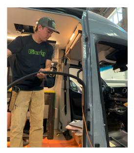
2C) Stop pulling when you reach the van floor. Tuck gasket under van and out of the way.
