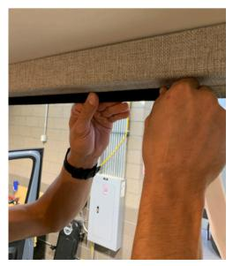
3H) When you get to the left side upper corner the velcro will want to pull away from curve. You will need to cut relief cuts and press back into place.
