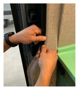
3I) When you get to the bottom, pull the tape down to. Determine the cut point at the bottom of the pillar. Trim to fit your van floor. You will have extra tape.
