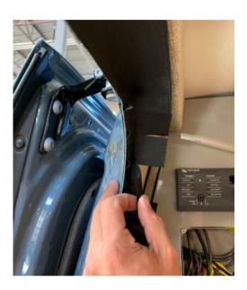
4G) Press the velcro in place down to the step. Trim the velcro at the lowest point and press it into place.
