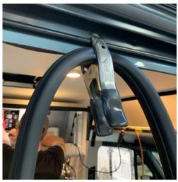
**DO NOT USE** a rubber mallet to secure the gasket during this phase. Instead, use only your hand to press it into place. Using any tool other than your fist may damage the gasket. The mallet will be utilized at a later stage.
