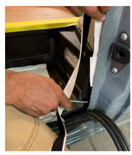
3E) Pull tape up to top of pillar and slide in to place w/o taking backer off. While removing backing about 6"to 8" at a time, press velcro in place maintaining the edge of the velcro and door trim.
