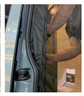
6J) Attach door sweep so no void can be seen at step. You may move this up and down to get a good seal.
