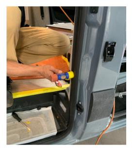
5J) Just after the first curve, stop and put a spring clamp. Move up to roof spring clamp and work from there to corner. Use the hook tool to get through corner. Continue down to spring clamp. Follow up with mallet to secure gasket.
