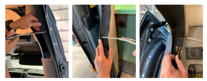
4G) Press the velcro in place down to the step. Trim the velcro at the lowest point and press it into place.
