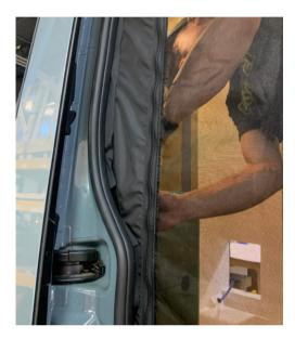
6K) Screen should close completely down right side with magnets and should have no voids. If void is seen, then adjust velcro piece to insure proper fit.
