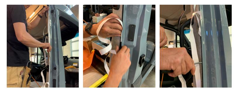
3G) As you work up to the corner you will have little humps of velcro on inside curve. This is ok as they will be trimmed later. Continue along top of door to left corner.
