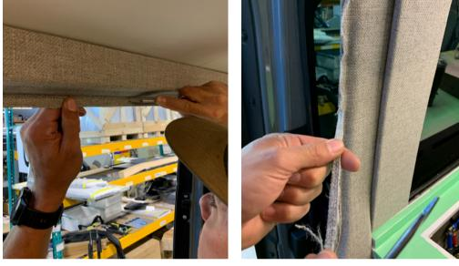
3D) Grab the 3/4"velcro with white peel off backer and peel back 1"-2" of backer and slide into lower right side slot. Using a screwdriver, slide velcro into slot and begin to peel back white backing while working your way up pillar. You may have to peel off and reset, which ok.
