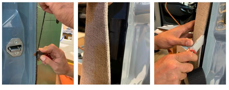
3M) Place 2" auto masking tape on fabric pillars. This will make it easier in the next step not to have velcro stick to the fabric. Skip this step if your van has plastic pillars.
