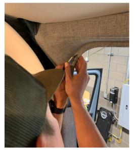
3C) Using a screwdriver will help work the fabric off.
