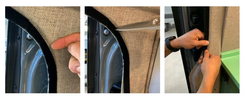
3I) When you get to the bottom, pull the tape down to. Determine the cut point at the bottom of the pillar. Trim to fit your van floor. You will have extra tape. Press the remaining into place and use tool if needed to make sure it's adhered.
