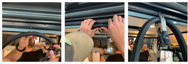
**DO NOT USE** a rubber mallet to secure the gasket during this phase. Instead, use only your hand to press it into place. Using any tool other than your fist may damage the gasket. The mallet will be utilized at a later stage.
